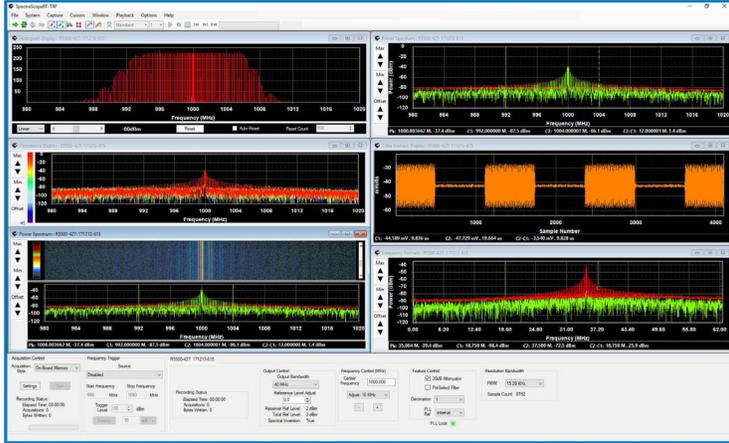
SpectraScopeRT is a Windows based spectrum analyzer application that requires no programming and allows for integrated operational control of both the downconverter receiver and the digitizer for signal capture, analysis, recordings. Any tuner, downconverter, or receiver with an IF output or a virtual receiver is supported.
