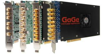
External multi-channel Digitizers with 16-bit A/D sampling rates up to 500 MS/s are available for use with the DCA08G or DCA27G Downconverter models. The large onboard FIFO memory of the external Digitizers allows for real-time streaming of I and Q baseband signals via PCI Express (PCIe) to the controller's memory for post processing, display, and storage.
